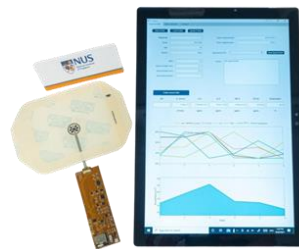
Fig -3: The VeCare platform is made up of four key components positioned in a clockwise direction from the bottom left: a chip, a wound sensor, a bandage, and an app. Together, these components enable real-time and point-of-care monitoring of chronic wounds.
